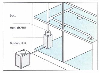
[The air handling unit can be connected to ductwork that runs throughout the house.]
